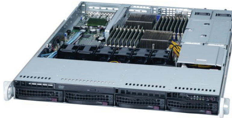
FIGURE 2 1U server: notice that the airflow is always obstructed
