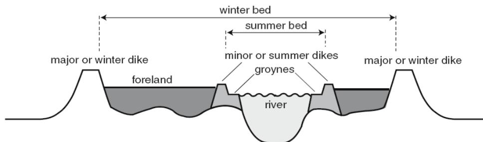
**Figure 3.5 Cross-section of the large rivers of the Netherlands (De Vaate et al., 2006)**
