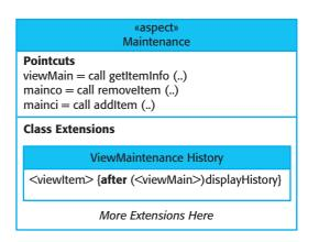
Figure 21.15 Part of a model of an aspect
