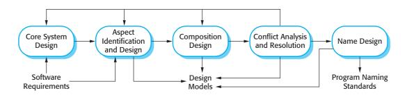
**Figure 21.13** A generic aspect-oriented design process
